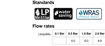
Flow rate data provided is indicative of each product and is given in open outlet conditions. Installation design, external connections and fittings not supplied may affect the data provided.
